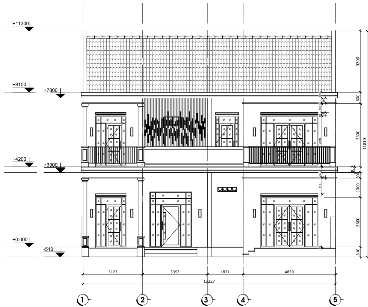
SCALE 1/120 ELEVATION-FRONT (WITHOUT GATE)
